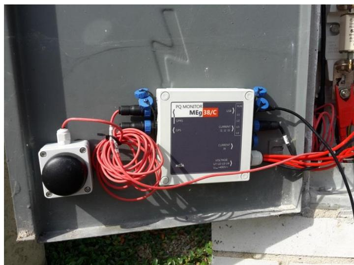
Figure 18 - Meg38 power quality measurement device with GPRS/LTE
