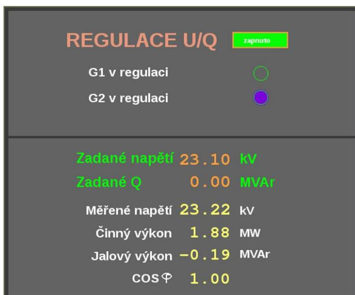
Figure 24 - CEZ Distribuce DMS (SCADA) - command tool for volt-var control for small hydro Vydra 6.4 MW
