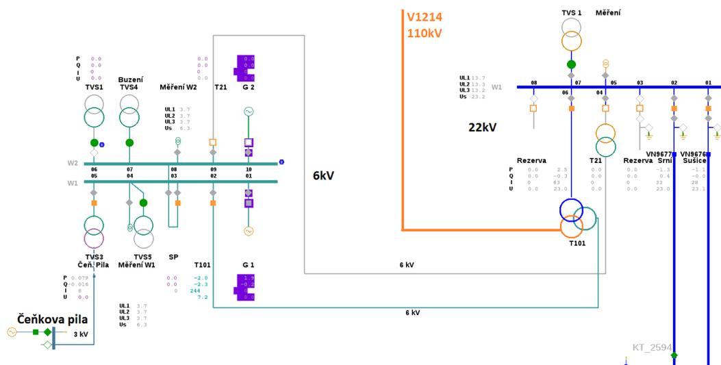
Figure 22 - Single line diagram for small hydro Vydra 6.4 MW connected to the HV or MV distribution network
