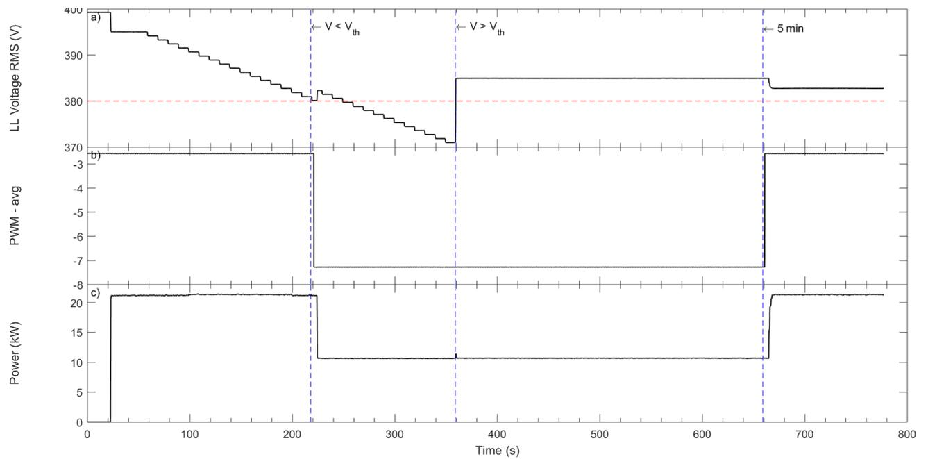
Figure 22 EVLink Parking – response to voltage sweep.
