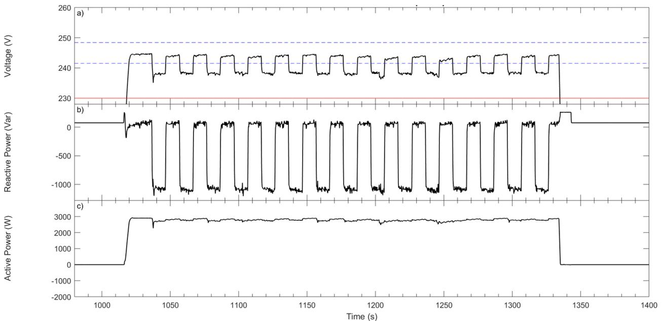
**Figure 12 Conext RL 3000 – response to voltage step. Worst case scenario – both additional impedance and steep droop curve.**
