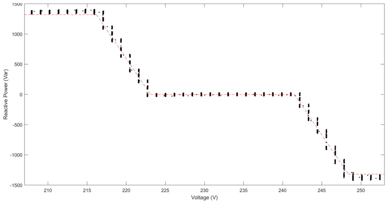
**Figure 7** Conext RL 3000 – response to voltage sweep. Droop characteristic.  $P = 80\%$  of the nominal apparent power. The setting for  $Q_{max}(\%)$  was increased to 53% from the previous value of 44%
