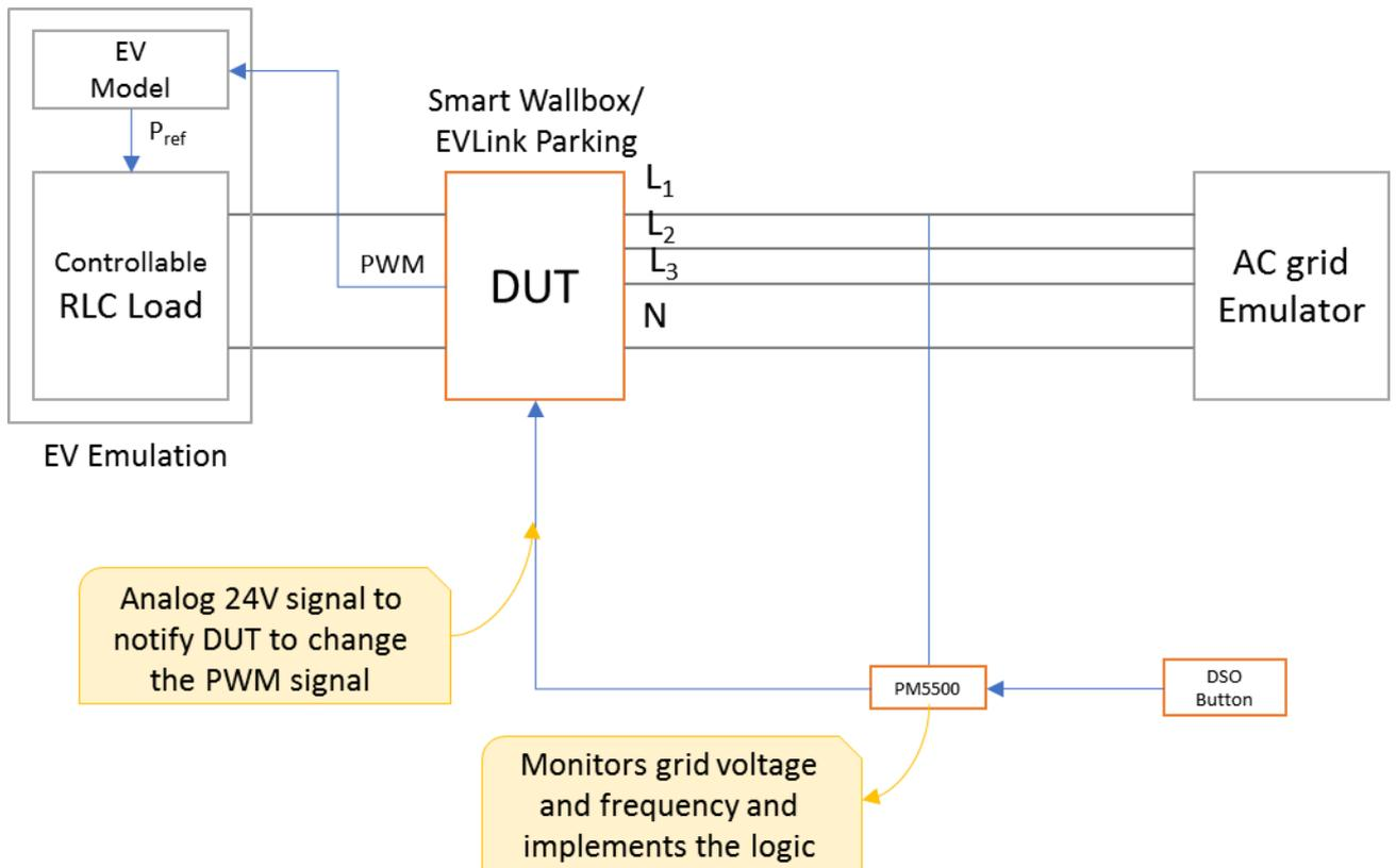
Figure 17 Diagram of the laboratory setup used for evaluating the *Smart Wallbox* and the *EVLink Parking* three phase EV charging station.
