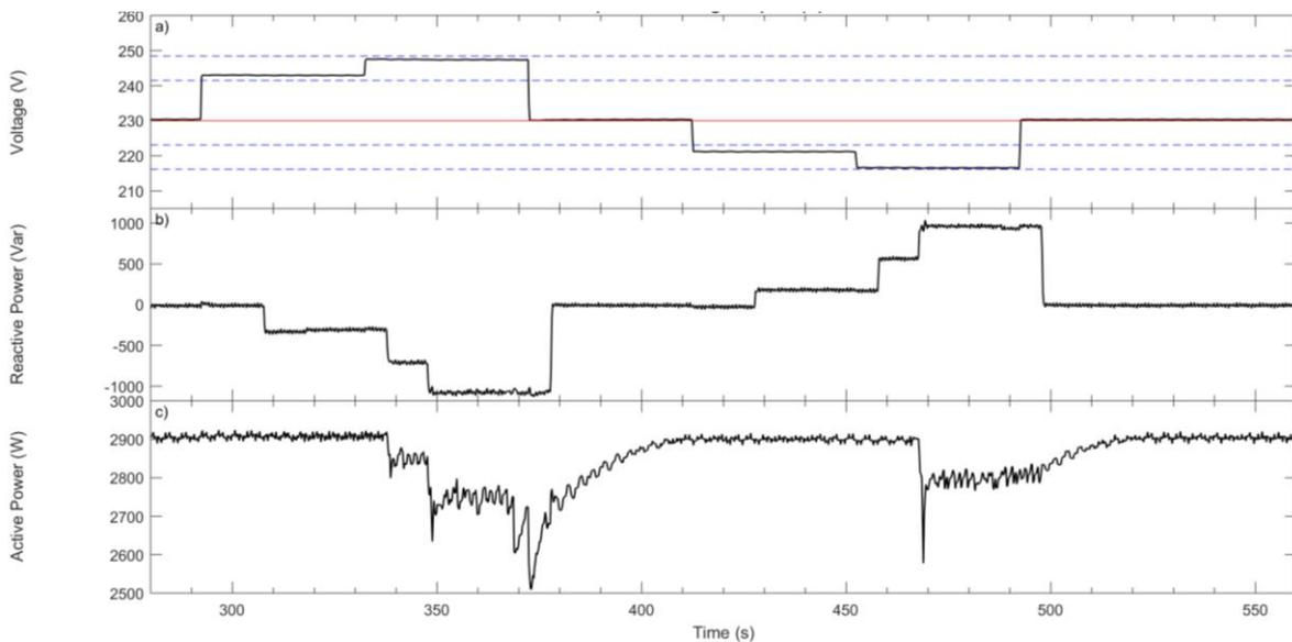
Figure 9 Conext RL 3000 – response to voltage steps. P = 100% of the nominal apparent power.
