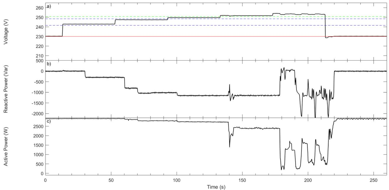
**Figure 16 Conext RL 3000 – response to voltage steps. P(U) enabled. P = 100% of the nominal apparent power. Unstable response.**
