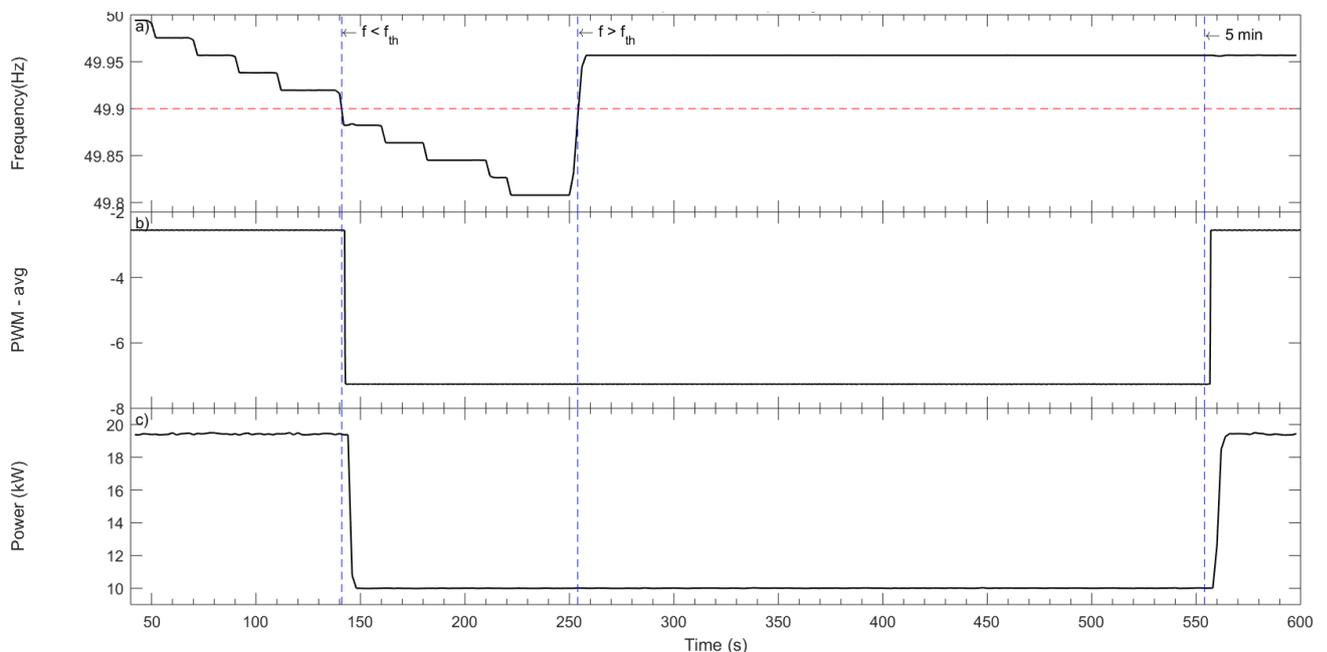
Figure 18 Smart Wallbox – response to frequency sweep.
