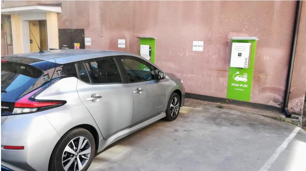
Figure 40- Smart charging stations in Hradec Kralove area provided by Schneider Electric (each with 1 x Mennekes connector 3x32A/400V + home socket 1x10A/230V)
