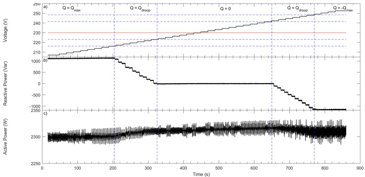
**Figure 2 Conext RL 3000 – response to voltage sweep. Voltage, reactive power, and active power time series. P = 80% of the nominal apparent power.**
