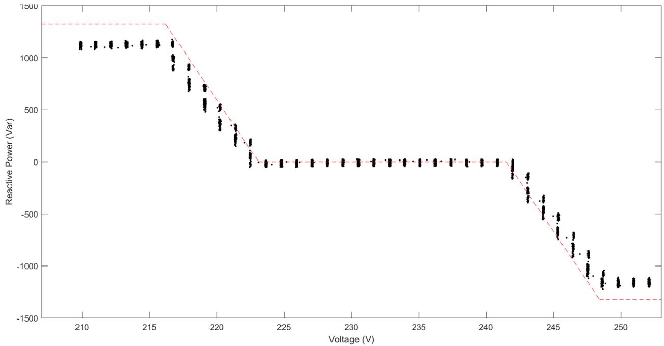
**Figure 5 Conext RL 3000 – response to voltage sweep. Droop characteristic. P = 100% of the nominal apparent power.**
