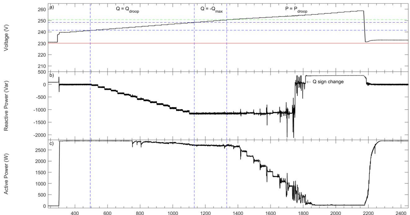
**Figure 13 Conext RL 3000 – response to voltage sweep. Voltage, reactive power, and active power time series. Both Q(U) and P(U) controllers are enabled. P = 100% of the nominal apparent power.**
