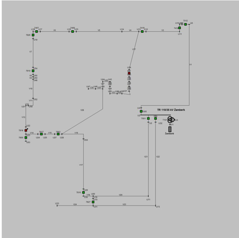
Figure 30 - Topology of MV distribution network where PV Zamberk 1.1 MWp is connected
