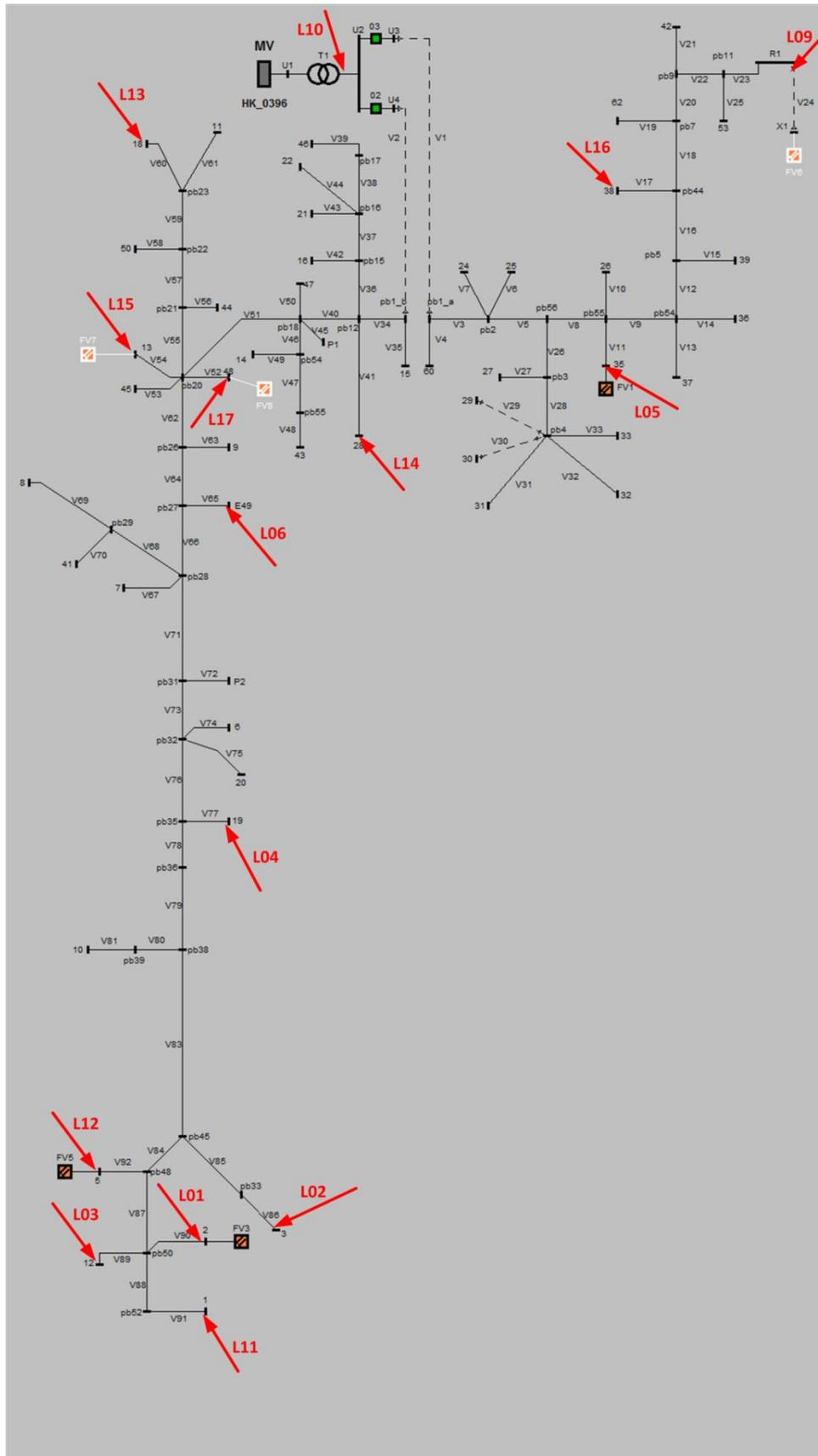
Figure 47 -LV grid topology in Luzany area (DNCalc model) with marked places for installation power quality measurement devices (red arrows)
