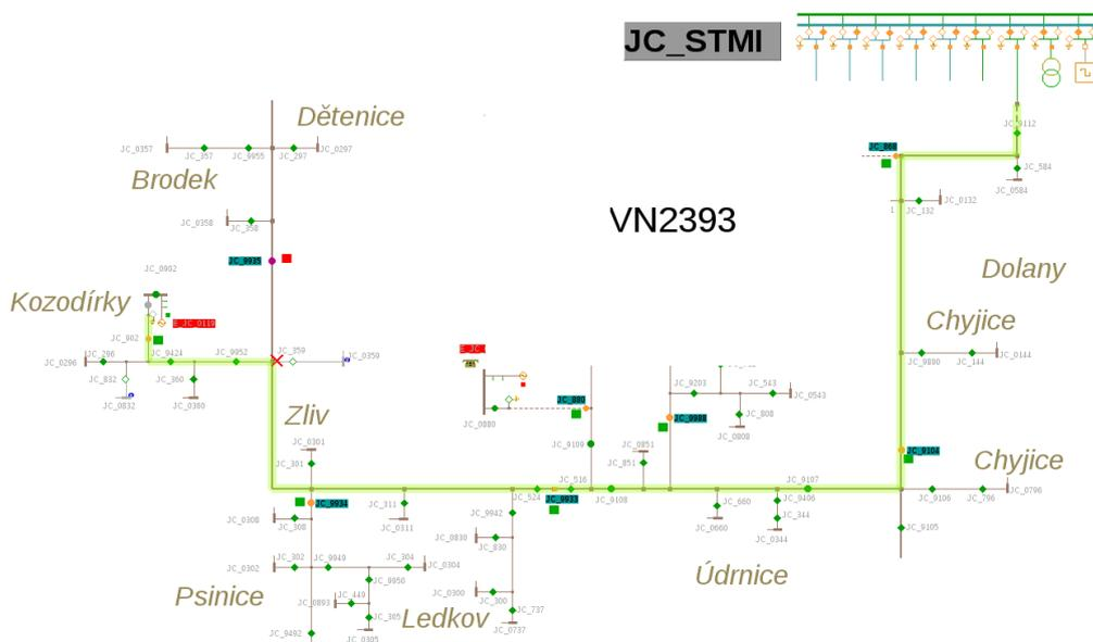
Figure 38 - Single line diagram for biogas station Detenice 1.25 MW connected into the MV distribution network
