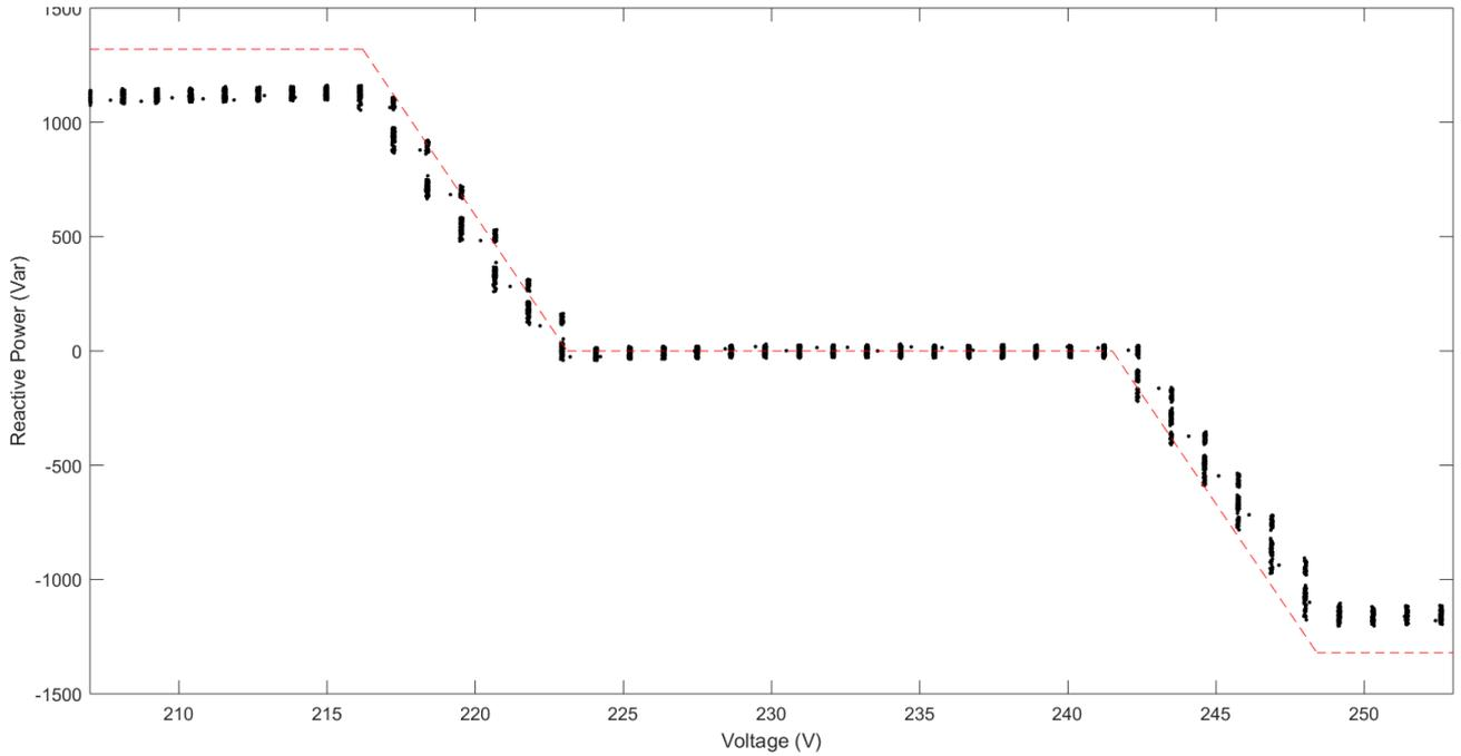
**Figure 3 Conext RL 3000 – response to voltage sweep. Droop characteristic. P = 80% of the nominal apparent power.**
