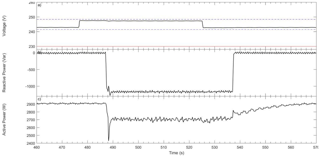
**Figure 11 Conext RL 3000 – response to voltage step. Worst case scenario – steep droop curve. The voltage at which the droop starts was set to  $V_3 = 244V$  and the voltage at which the droop saturates was set to  $V_4 = 246V$ .  $P = 100\%$  of the nominal apparent power.**
