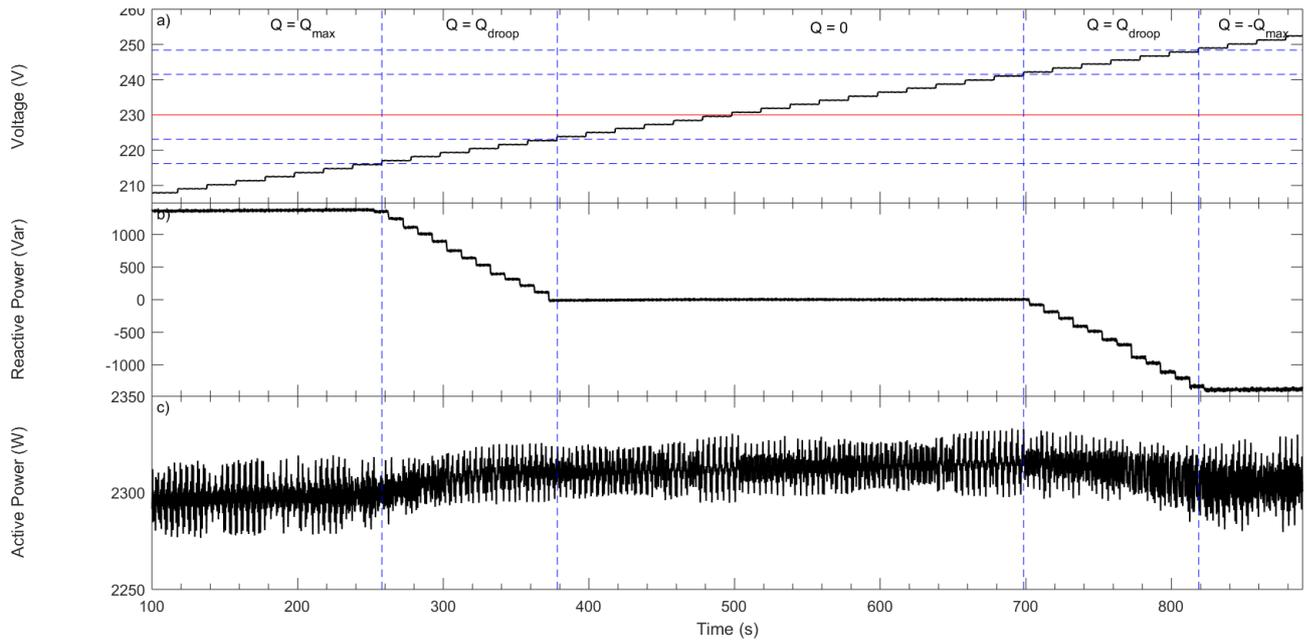
**Figure 6** Conext RL 3000 – response to voltage sweep. Voltage, reactive power, and active power time series.  $P = 80\%$  of the nominal apparent power. The setting for  $Q_{max}(\%)$  was increased to 53% from the previous value of 44%
