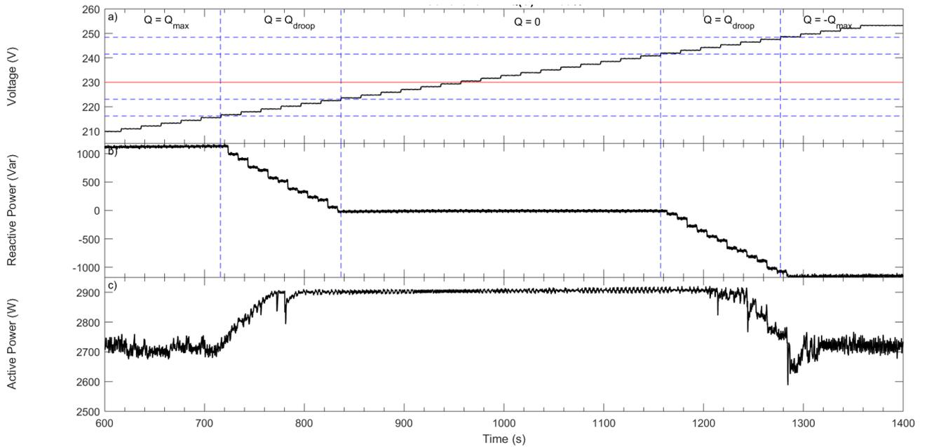
**Figure 4 Conext RL 3000 – response to voltage sweep. Voltage, reactive power, and active power time series. P = 100% of the nominal apparent power.**
