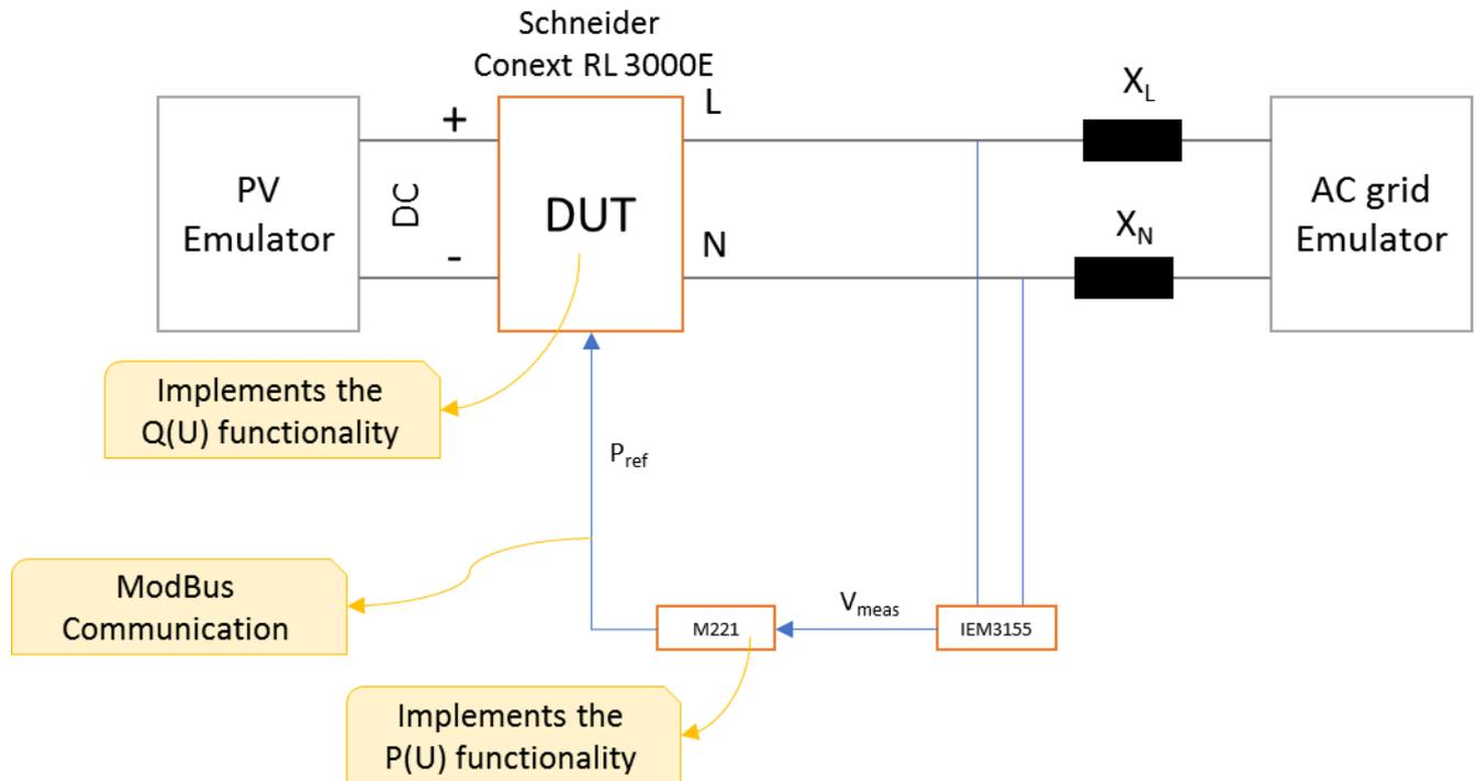
Figure 1 Diagram of the laboratory setup used for evaluating the Schneider Conext RL 3000 single phase PV inverter.
