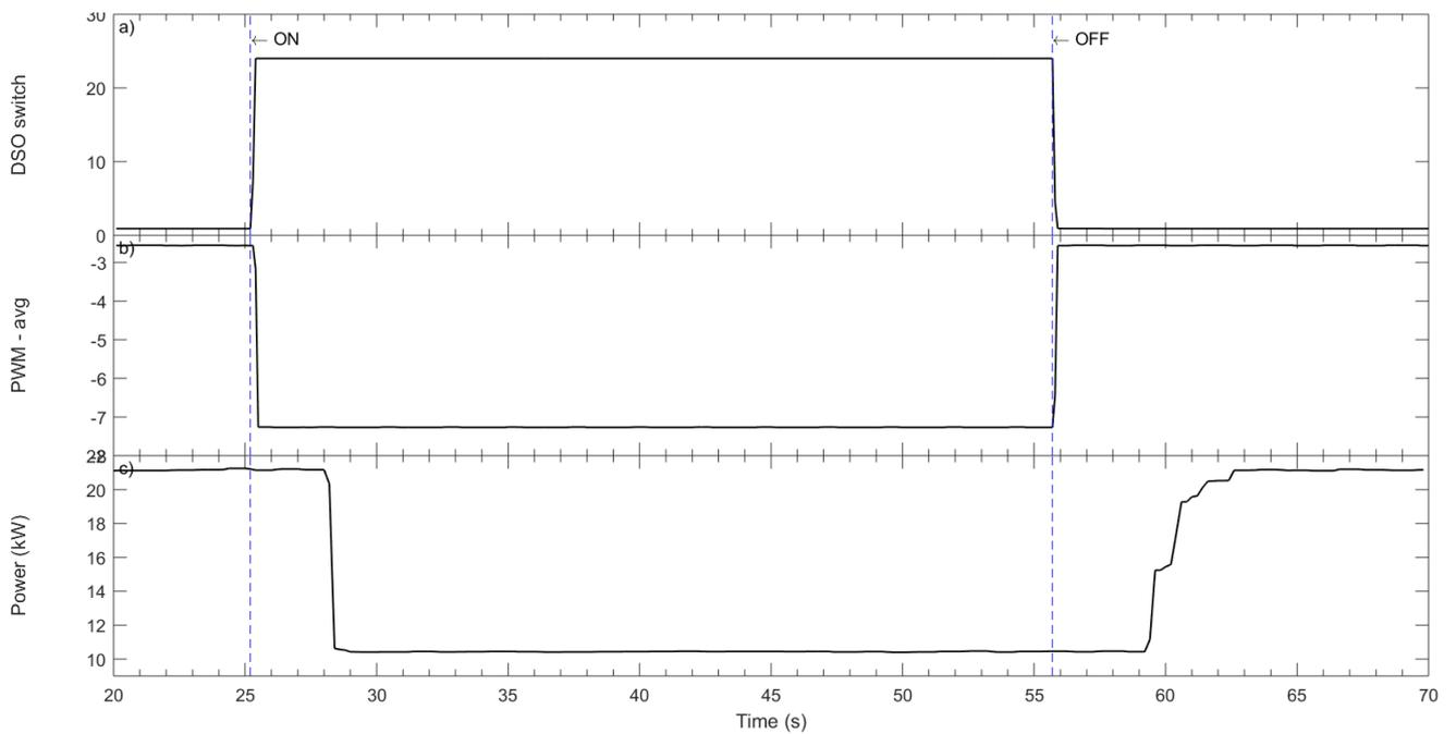
Figure 20 Smart Wallbox – response to DSO switch.
