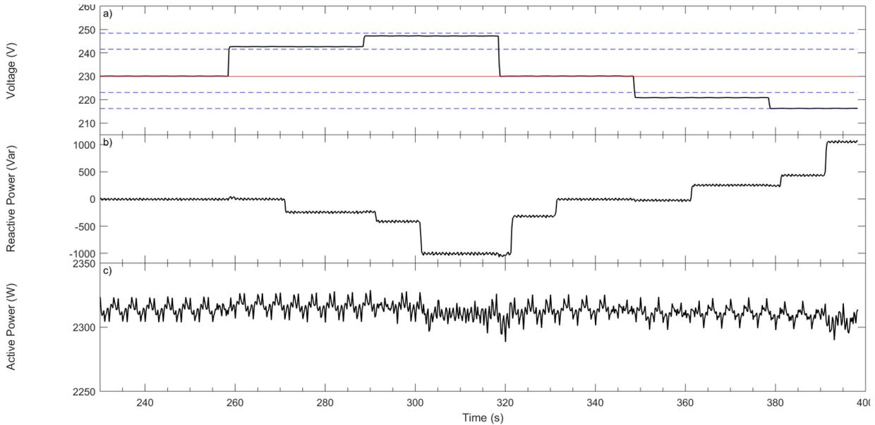
Figure 8 Conext RL 3000 – response to voltage steps. P = 80% of the nominal apparent power.
