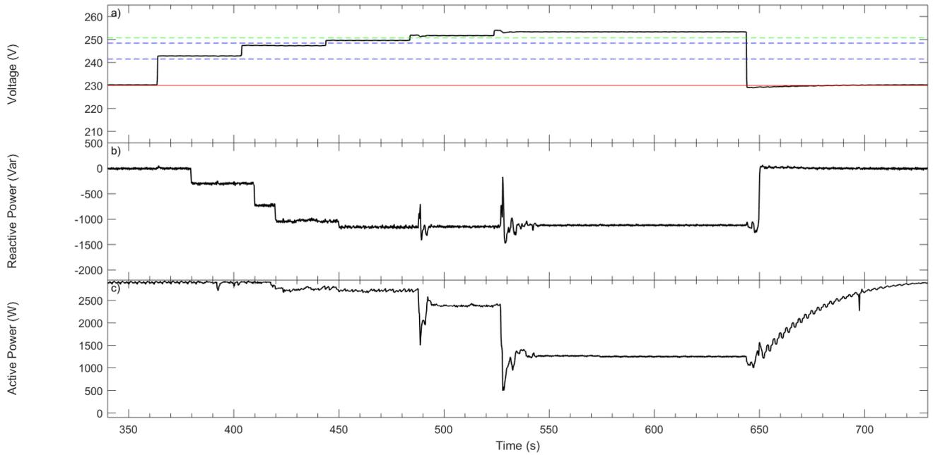
**Figure 15 Conext RL 3000 – response to voltage steps. P(U) enabled. P = 100% of the nominal apparent power. Stable response.**
