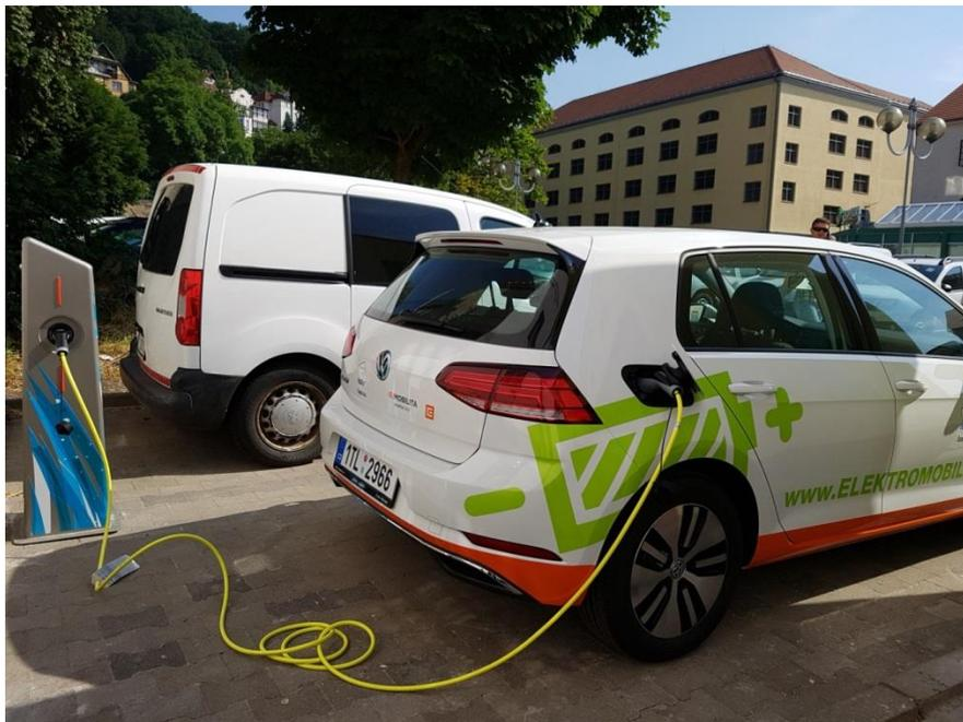
Figure 42- Smart charging station in Decin area provided by Siemens with 2 x Mennekes connectors (with 3x32A/400V each)
