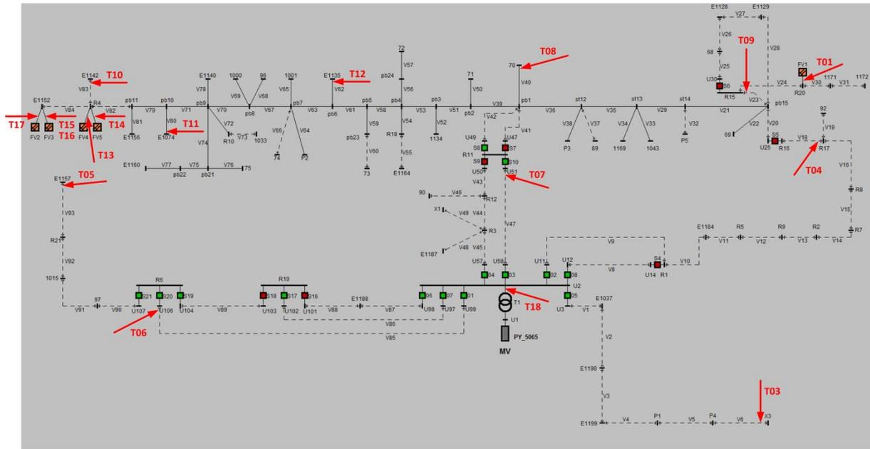
Figure 12 - Use case WP6\_1 - LV grid topology in Teptin area (DNCalc model) with marked places for installation power quality measurement devices (red arrows)
