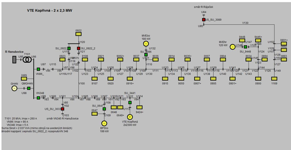
Figure 36 - Topology of MV distribution network where wind park Koprivna 4.6 MW is connected (DNCalc model)
