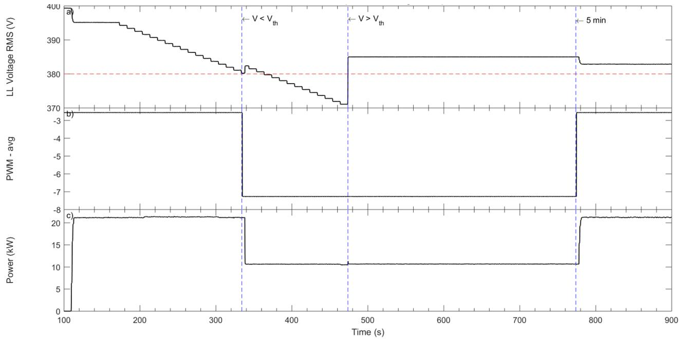
Figure 19 Smart Wallbox – response to voltage sweep.
