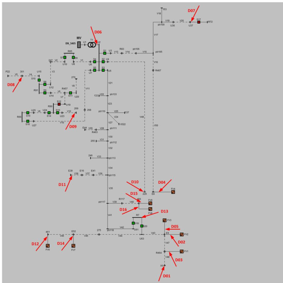
Figure 8 - Use case WP6\_1 - LV grid topology in Divisov area (DNCalc model) with marked places for installation power quality measurement devices (red arrows)
