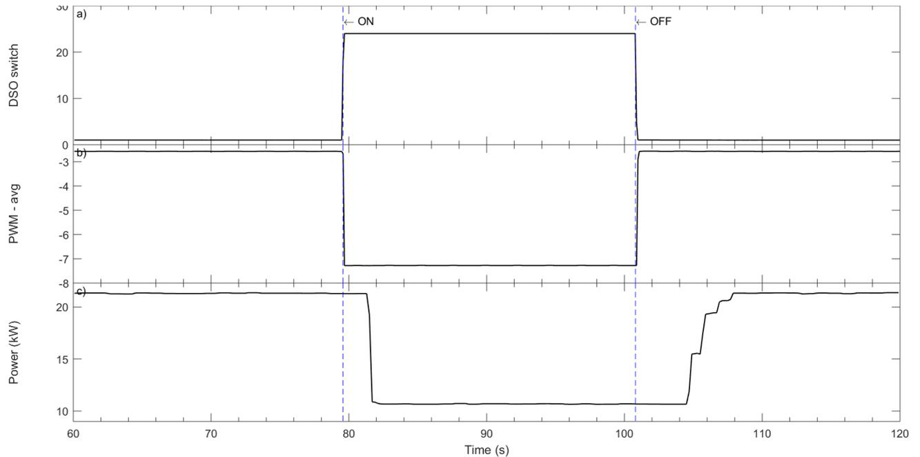
Figure 23 EVLink Parking – response to DSO switch.
