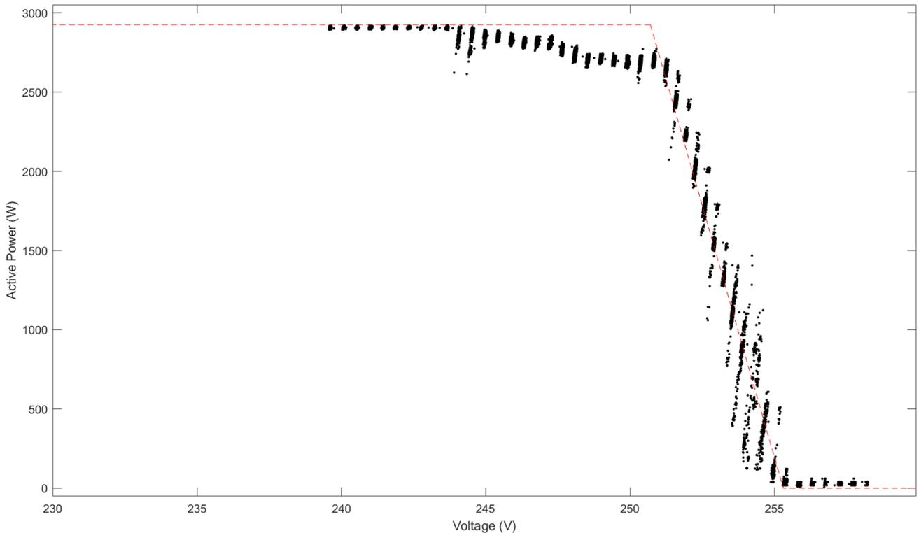
Figure 14 Conext RL 3000 – response to voltage sweep. P(U) droop characteristic.
