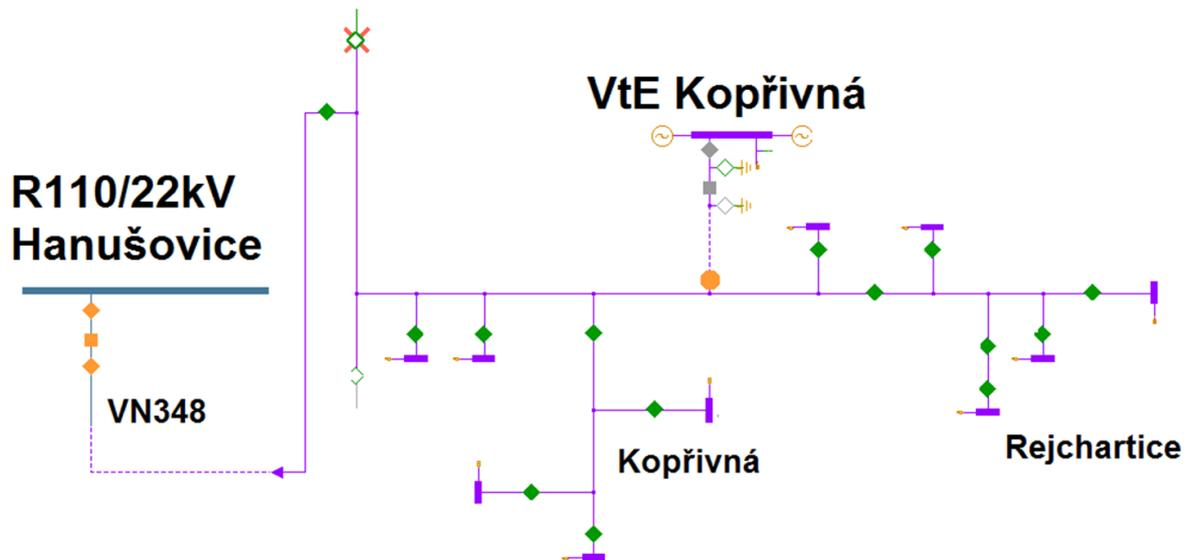
Figure 33 - Single line diagram for wind park Koprivna 4.6 MW connected into the MV distribution network
