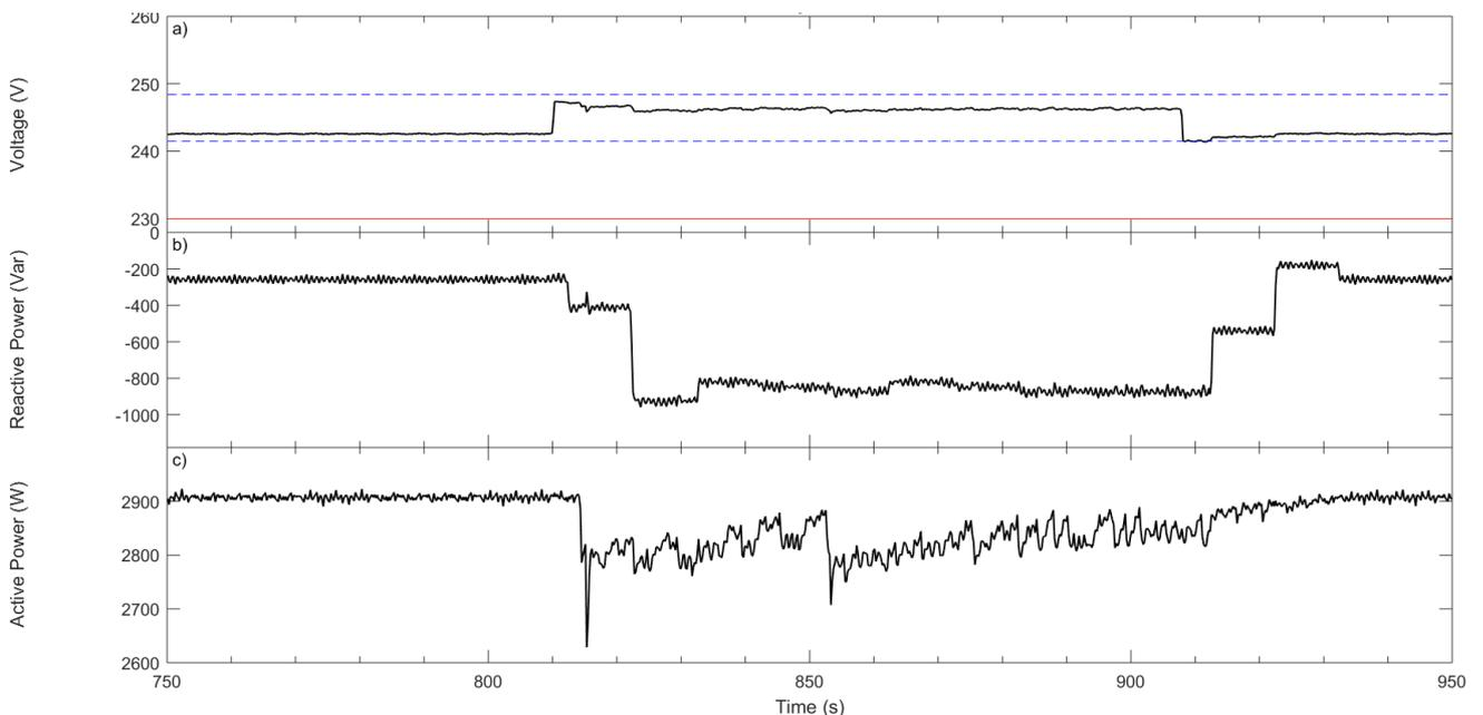
**Figure 10 51 Conext RL 3000 – response to voltage step. Worst case scenario – additional impedance between the inverter and the grid simulator  $X = 0.387 + i1.019$ .  $P = 100\%$  of the nominal apparent power.**
