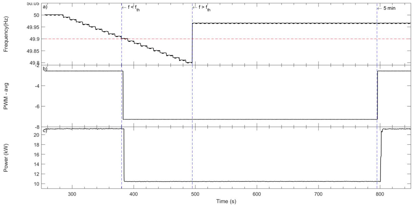
Figure 21 EVLink Parking – response to frequency sweep.
