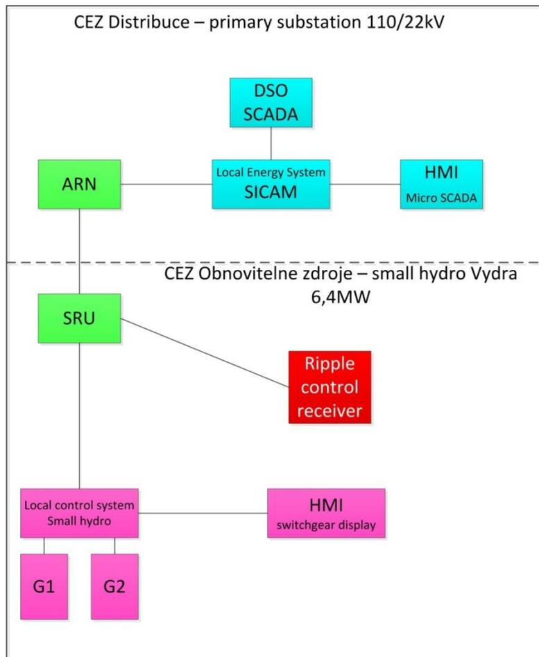
Figure 25 - Topology of control systems for volt-var control at small hydro Vydra 6.4 MW
